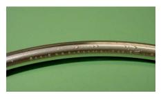
**Figure 1:** Blisters seen on a standard silver plated seal after 1,000 hours in air at 500°F
