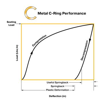
**Springback:** The difference between the working height and the (reduced) free height after all applied loads have been released: this represents the total elastic recovery of the seal.
