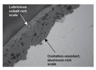
**Figure 2:** TriCom-HT forms a multi-layer oxide scale at service temperatures to simultaneously slow oxidation and wear.
