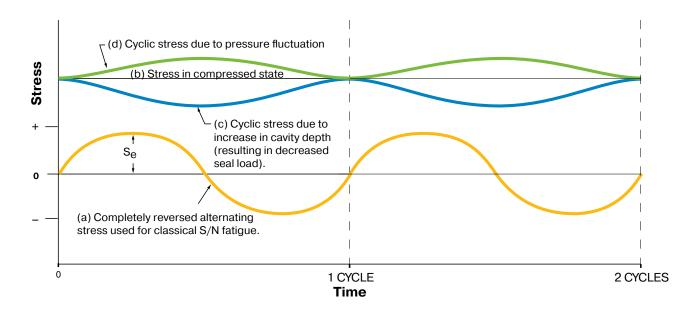
There are several types of loading that can result in fatigue failure, the most common type being alternating tension and compression or reversed loading. Loading of this type is illustrated in line (a) in the figure above, and is the type used in fatigue testing to develop the endurance or fatigue limits  $(S_e)$  of materials. The endurance limit is the stress below which fatigue failure will not occur, regardless of the number of applied cycles (generally considered  $10^7$  cycles).
