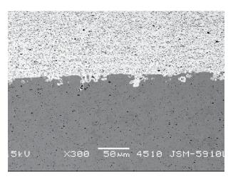
**Figure 1:** TriCom-HT is a composite coating consisting of a cobalt-nickel matrix with chromium carbide and MCrAIY reinforcing phases.
