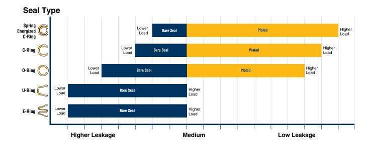
The graph above shows typical ranges of leakage rates that may be expected with various types of seals.
