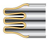
The customized **E-ring** can be designed with a large number and variety of convolutions. These seals provide exceptional springback when flange separation is of primary concern.
