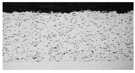
**Figure 1:** TriCom is a composite coating consisting of a cobalt matrix with chromium-carbide reinforcing phase.
